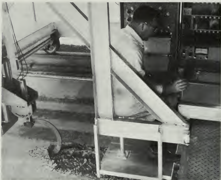
In research on tillage tools at the National Tillage Machinery Laboratory, Auburn, Ala., electrical signal outputs from electrical resistance strain gages, generators, and transducers are combined mathematically with transistorized analog computers, and final results are plotted by X-Y recorders.
